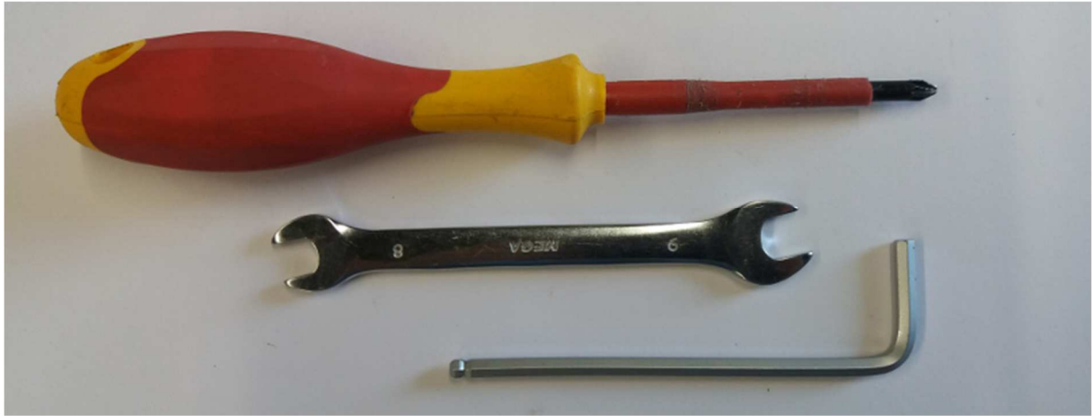
Fig. 79: The tools used in the assembly: Phillips screwdriver, bent Allen key M4, and wrench 8.
