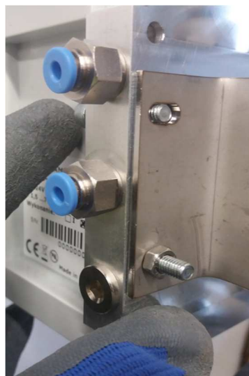
Fig. 86: Fitting positioner to the handles.
