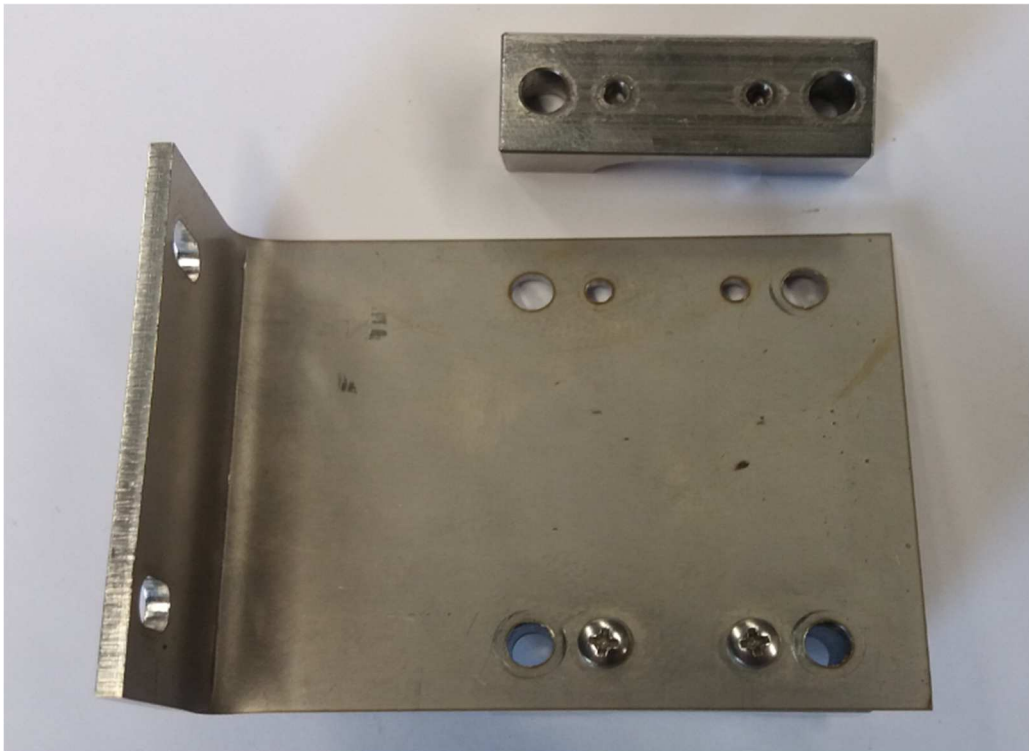
Fig. 82: Positioner handle with half of the clamp and screws M3x5.
