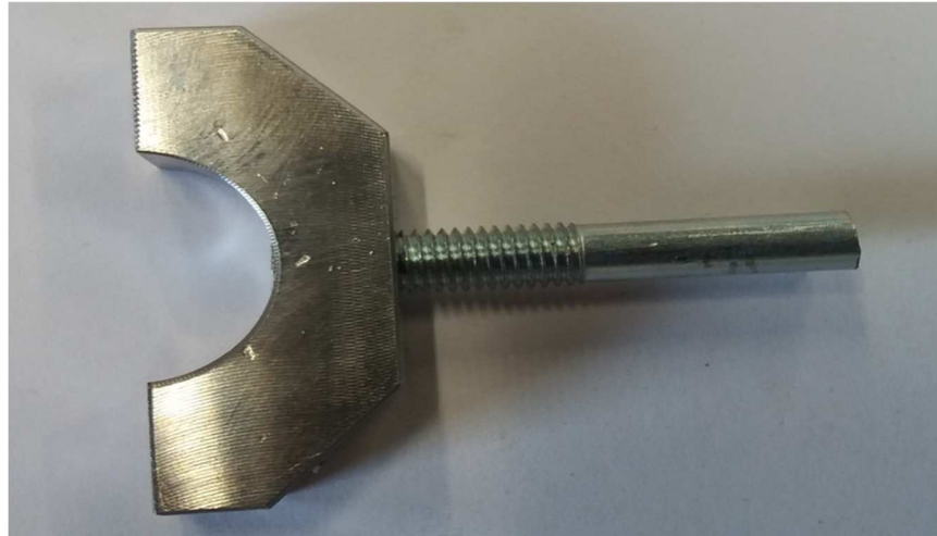
Fig. 81: Clamp of the stem with tightened screw.
