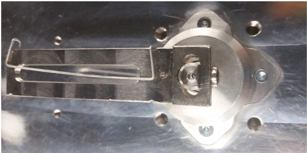
Fig. 80: The connection of positioner shaft with lever.
