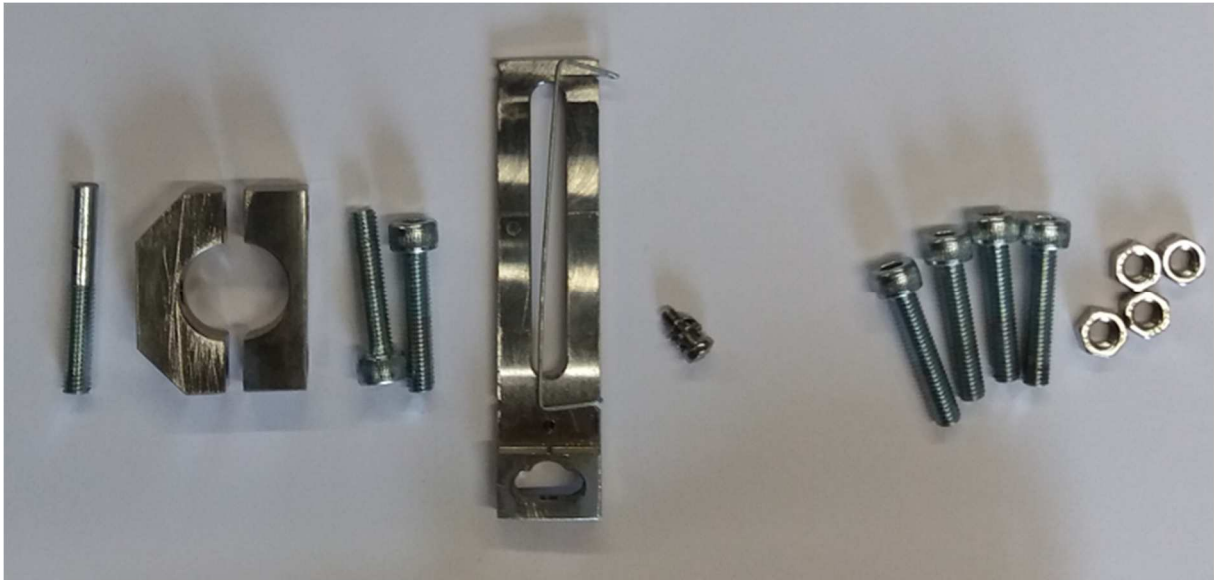
Fig. 77: From left: stem clamp with retaining screws, lever with spring and screw securing it to the positioner shaft, positioner mounting screws with handles.
