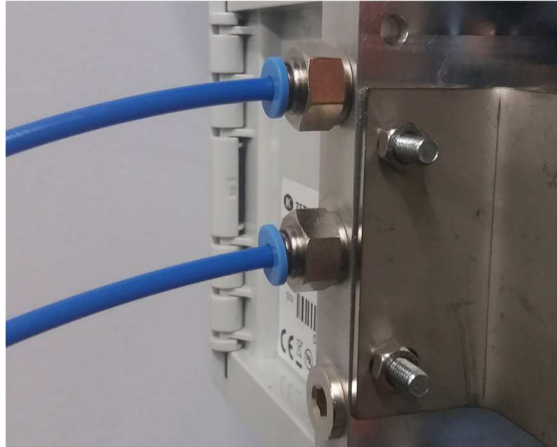
Fig. 92: Connecting the pneumatic valve (bottom) and the conductor of pressure (upper)
