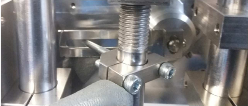
Fig. 90: Correct insertion of a screw coupling to the spring
